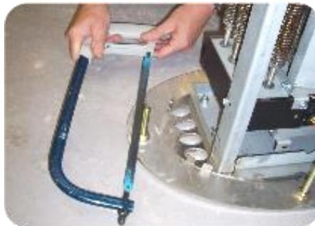
Remove only one M10 nut and refit and secure bolt with a stainless steel M10 dome nut supplied. Repeat for each of the other three projecting bolts one at a time. Both sections of the casing should be fitted only after all functional tests have been completed and verified (see Commissioning).
