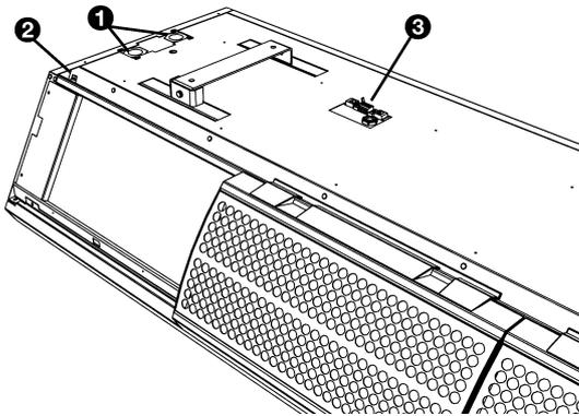
The air relief valve ② is located in the upper left of the unit.
