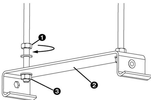
1. Fix four threaded rods M8 according to the dimensions in the table. Make sure the threaded rods are perpendicular.
