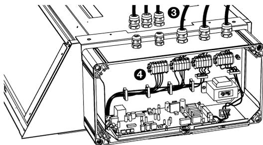
3. Lay the control cable(s) into the box, through the free cable gland(s) ③.
