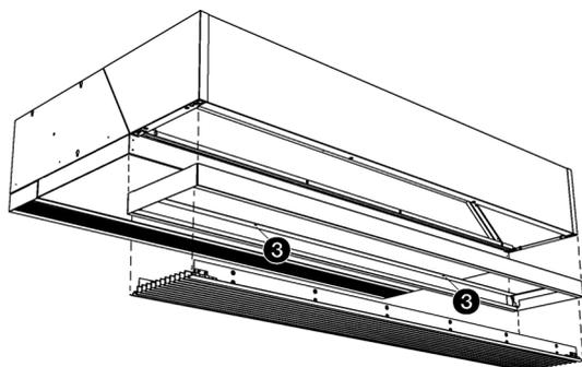
2. Loosen screws ❸ and remove the frame.
