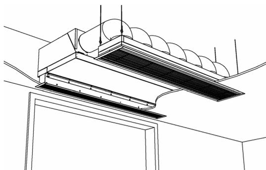
The recessed model is designed for integration into a false ceiling or into a cove, with the inlet opening possibly at some distance from the unit.
