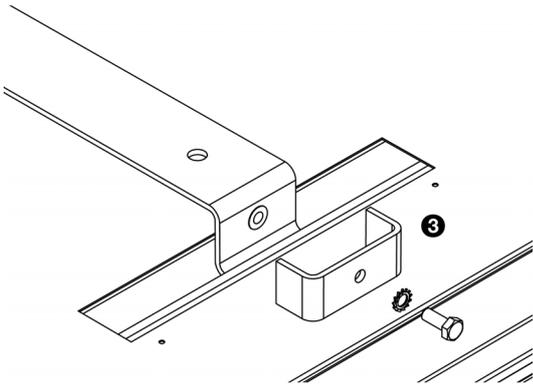
2. Fit a lock plate ③ to each suspension bracket.
