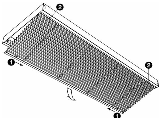
1. Remove the inlet grille from its frame:
