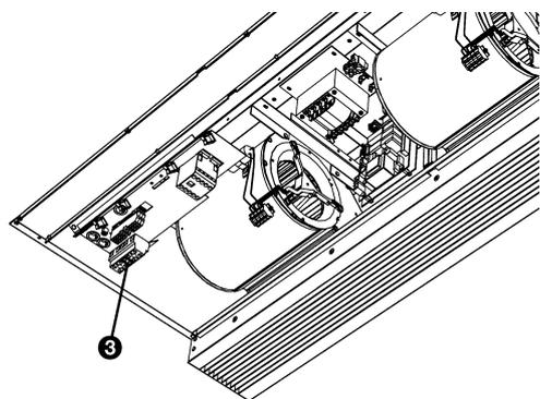
5. Connect the cable to the terminal ③ in the unit according to the wiring diagram.
