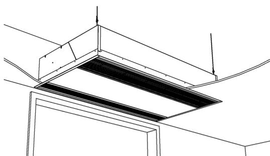
The cassette model is designed for installation above a false ceiling, with the inlet opening close to the unit and with easy access to the unit.
