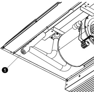
The drain plug ① is located on the left of the unit.
