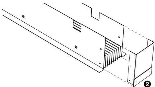
2. Install the end piece *without* finishing edge ②.
