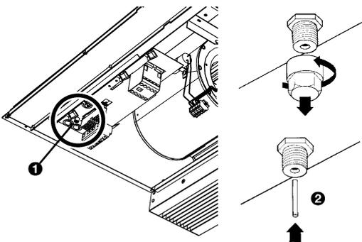
The unit is equipped with a maximum thermostat. This has to be reset manually if it trips.
